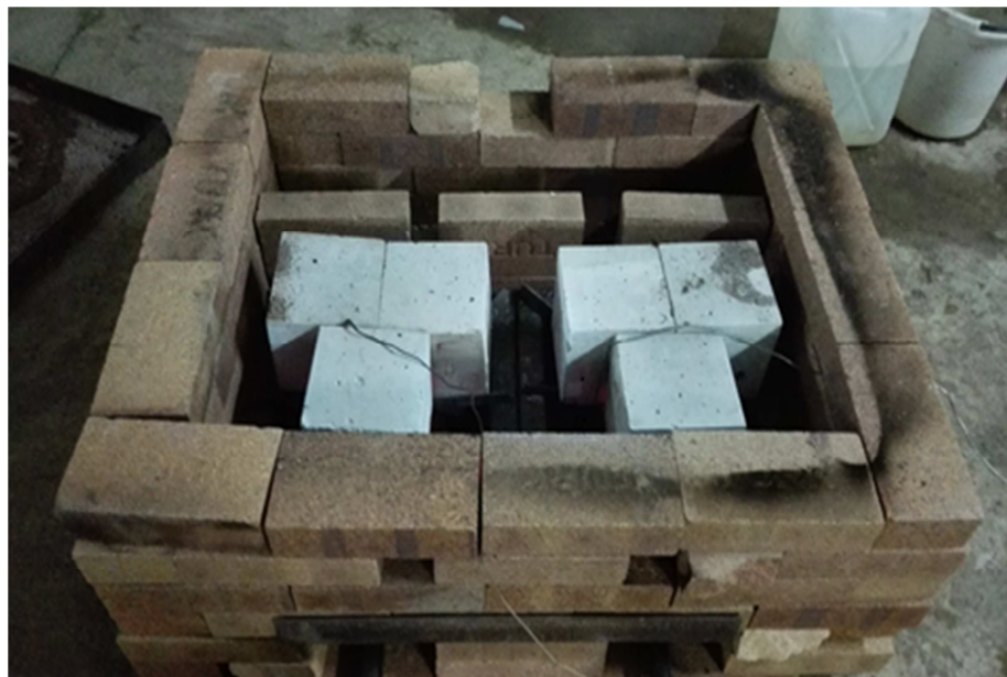
Figure 1: Firing furnace chamber
